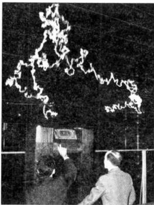
General Electric frequency modulation receiver undergoing comparative listening tests while subjected to million volt lightning discharge.
